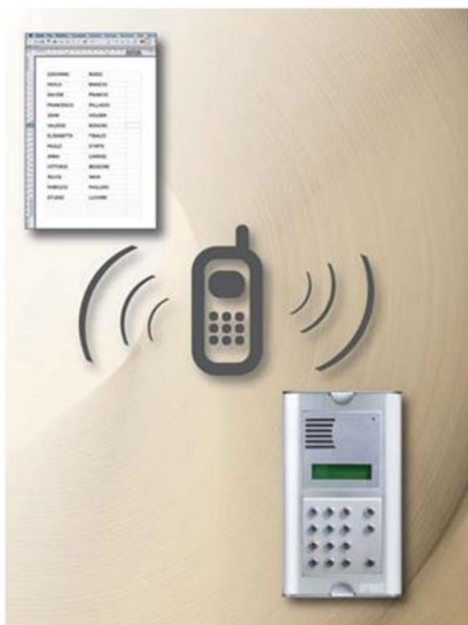
Easy name addition: using spreadsheet and sending data using a smartphone with Bluetooth connection (already fitted inside the entry panel).
