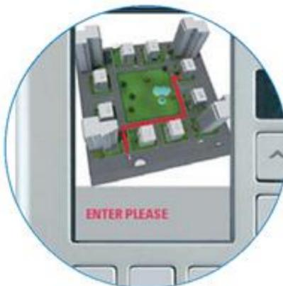
TFT 3.5" colour, with operation messages and guide for use. The display can also be used to leave audio/video messages if the called user is away and showing a map indicating how to reach the required building
